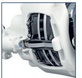
Covers can be installed during routine servicing or inspection of the disc brakes.
