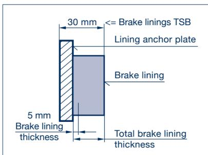
The thickness of the remaining pad must **NOT** be less than **5 MM**.
